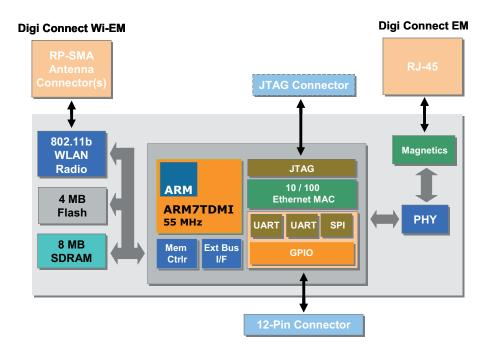
The Digi Connect EM and the Digi Connect Wi-EM are the industry's first interchangeable secure embedded modules, delivering wired and wireless Ethernet network connectivity that is cost-effective and easy to implement.
